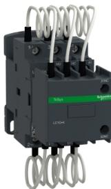
Capacitor contactor, TeSys D, 12.5 kVAR at 400 V/50 Hz, coil 220 V AC 50/60 Hz
